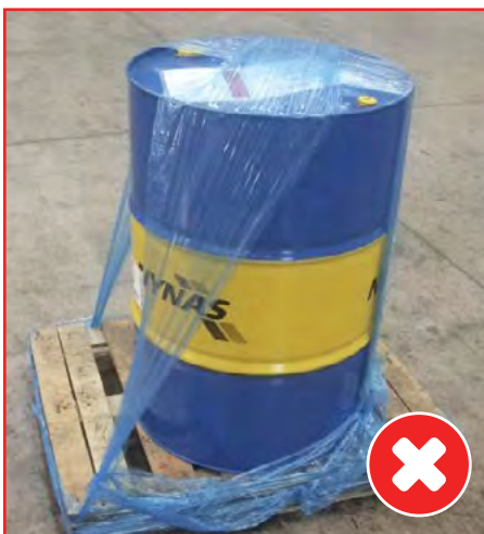
This drum is barely secured.
