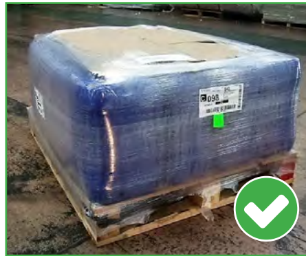
Drums, tied down and properly wrapped.
