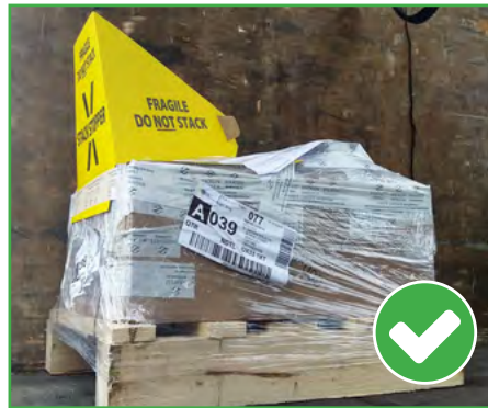
For fragile goods or micro pallets, use a stack stopper sign like this.
